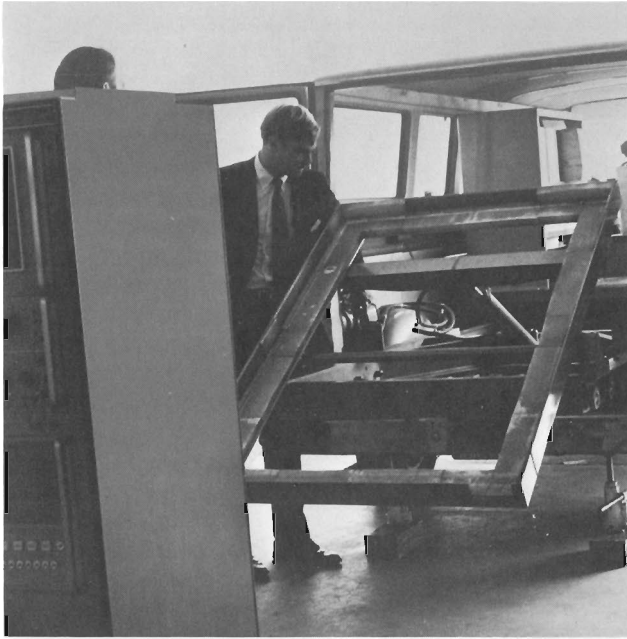
Urgent need for a device that would carefully load and unload demonstration network analyzer system resulted in this efficient rack operated here by Microwave's Jesse Pipkin. The equipment team delivered it eight days after order came in.
