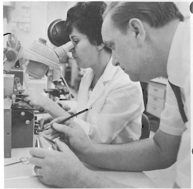
A microscope is required to operate "whisker bending" machine designed by Bill West, mechanical engineer. Here Bill uses giant model to demonstrate device for Marly Machado, who was able to handle machine with no prior training.
